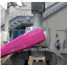
Pic. 12: Supporting position of the ACP on of the vice jaws
